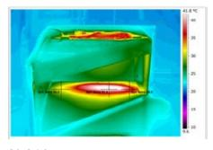
**41,4** °C Floor under Master Heater, middle **38,0** °C Floor under Master Heater, right side **34,0** °C Floor under Master Heater, leftside
