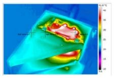
**41,9** °C Above the heating element **23,8** °C Left part above Master Heater **22,7** °C Next to Master Heater, front
