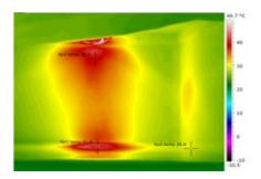
**41,8** °C Floor under the lamp **28,8** °C The right side from the lamp **39,3** °C Under the lamp/lid
